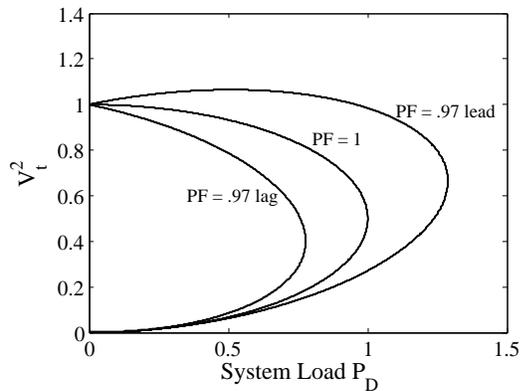
Figure 2. The “To” bus voltage of a small power system is plotted against system load. Loads with three different power factors are plotted.
