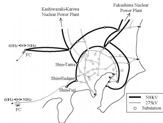
Figure 3. This is the layout of the 1987 TEPCO network. This figure is reproduced from reference [7].
