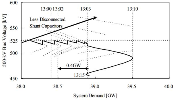
Figure 4. A visualization of TEPCO's Saddle Node bifurcation is plotted. This figure is reproduced from reference [7].
